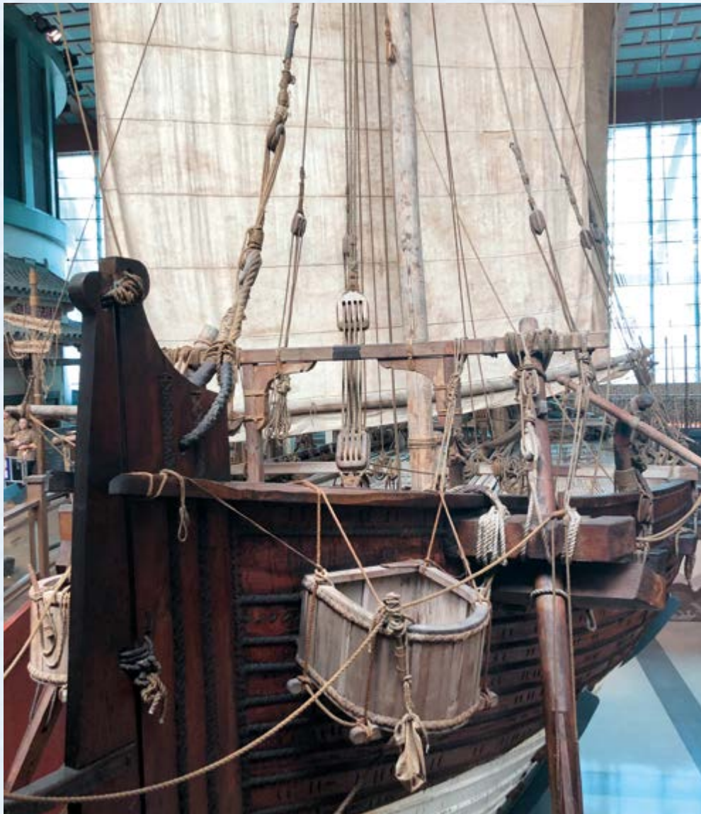
The Jewel of Muscat, a replica of the Tang era ship salvaged at Belitung was made in Oman and presented as a diplomatic gift to Singapore in 2010. Unlike most Arab dhows with triangular lateen sails, it has square sails. The original ship could have been made in India or the Arab Peninsula. It features a hull made of planks sewn with ropes made of vegetable fibre. This picture was taken when the Jewel of Muscat was housed at the Maritime Experience Museum at Sentosa, Singapore.
